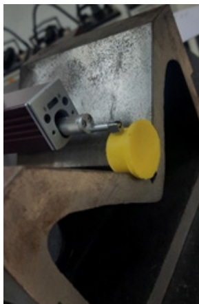
FIGURE 3. Surface roughness testing process.
