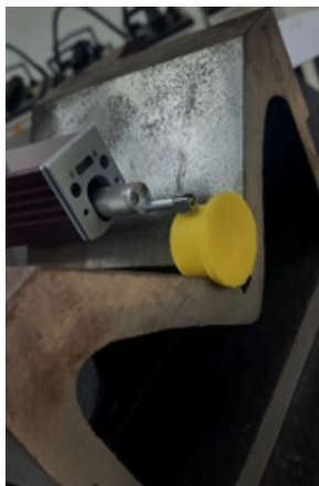
FIGURE 3. Surface roughness testing process.
