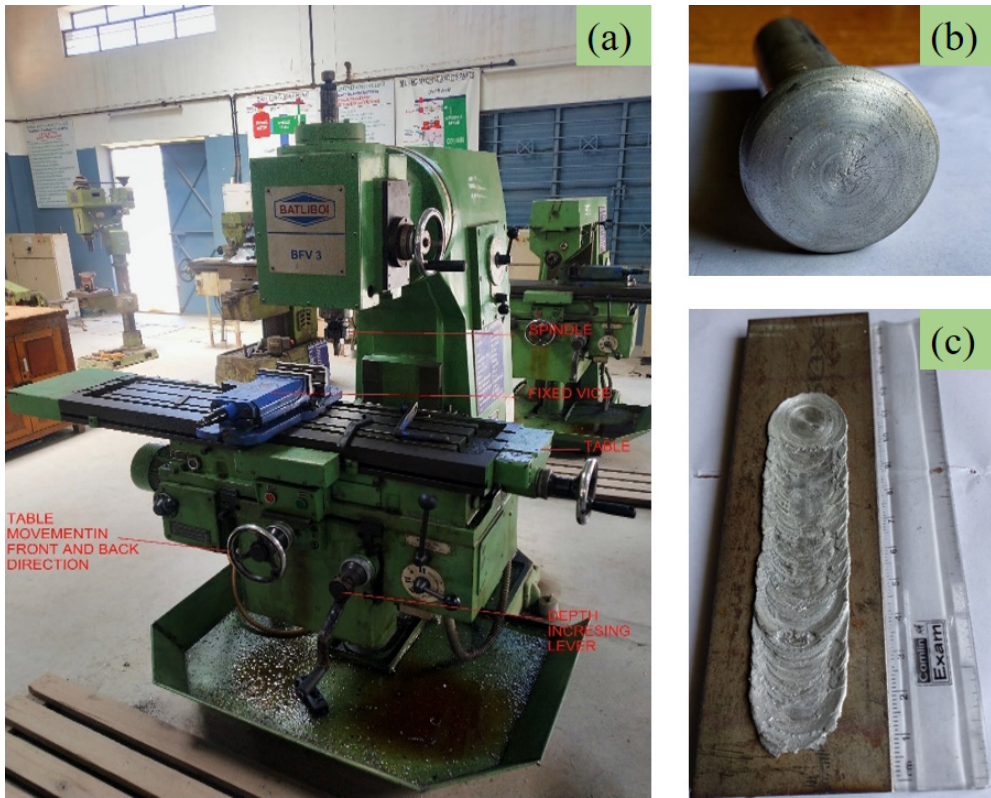
FIG. 1 (a) Vertical Milling Machine – Experimental Setup (b) Tool (c) Sample Specimen
